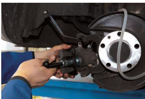
With floating calipers with an integrated parking brake (combined calipers), the piston must not simply be pushed back, as this would destroy the automatic adjustment mechanism in the caliper. In many cases the piston must be turned and pressed. This can be done using the ATE piston return tool set. With its right- and left threaded spindle and its 9 interchangeable adapters, it can be used for all common vehicles. It can also be used to return pistons in standard floating calipers.
