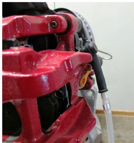
The ATE 90° adapter is a helpful accessory for bleeding in tight spaces. Thanks to its short design, the adapter is only 19 mm in size and allows brake fluid to be removed in spots which are difficult to access.
