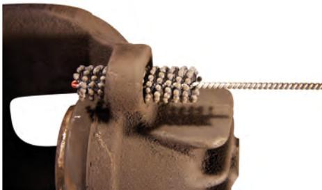
After some time of operation it may be useful to replace the (rubber) guide bushes in ATE floating calipers. The mounting hole in the caliper housing is often corroded to a greater or lesser degree. This will cause the guide bushing to be squashed and the guide pins may become jammed in them. This will restrict brake caliper movements which may lead to other braking problems.
