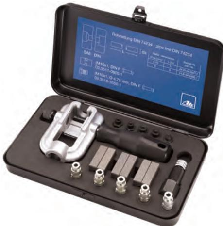
ATE's handheld pipe flaring unit is a low-cost piece of equipment for the quick and uncomplicated flaring of 4.75 mm, 5 mm and 6 mm diameter brake pipes to Shapes E and F in conformity with DIN 74234 / ISO 4038.
