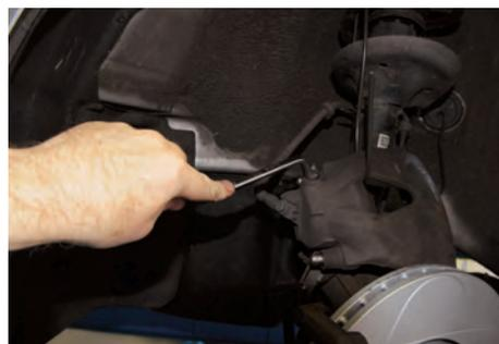
The special ATE bleed wrenches are ring wrenches with an internal hexagonal head to prevent the damage of bleed valves. Thanks to a long offset and a short offset, they can be used without removing the wheel.
