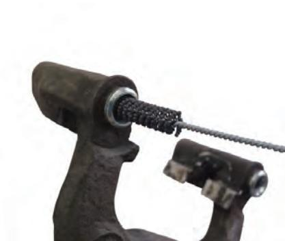
Lubricated guide pins are used to hold the "LUCAS" floating calipers in place. Rubber bellows provide the pin seal. Damaged bellows will make the guide bushes inside the brake caliper holder corrode. This will restrict caliper guide movements and may lead to additional braking problems.
