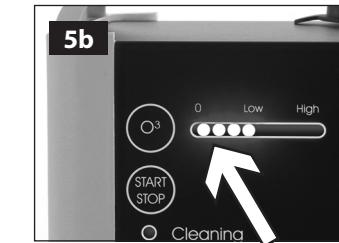
**EN** LED lighted on 'Low' position. Ozone treatment 15 min. Immediately after this ozone treatment, the treatment with the Air Purifier liquid will start. This position is chosen for strong smell problems.
