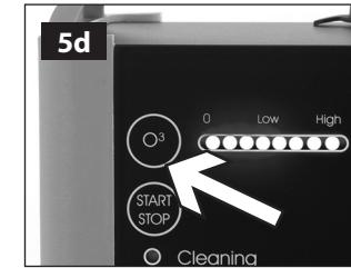
If the LED light is in 'High' position and the O<sub>3</sub> button is pushed, it moves to 0 position.
