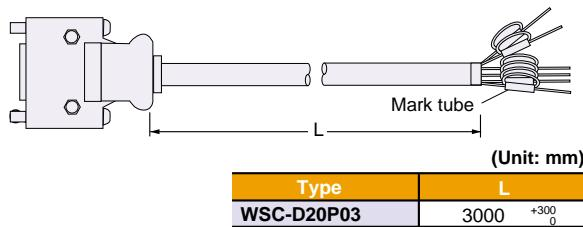
**Series:** Option cable for input/output of control signals
