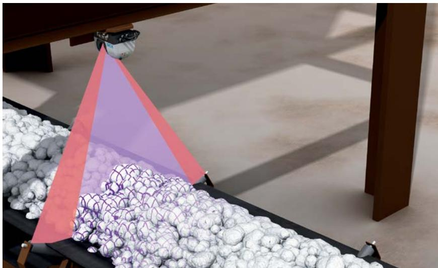
Shifting of the conveyor belts can sooner or later lead to belt wear. Bulkscan® LMS511 detects the loading position and limit at an early stage using the belt monitoring function. This ensures optimal system utilization.
