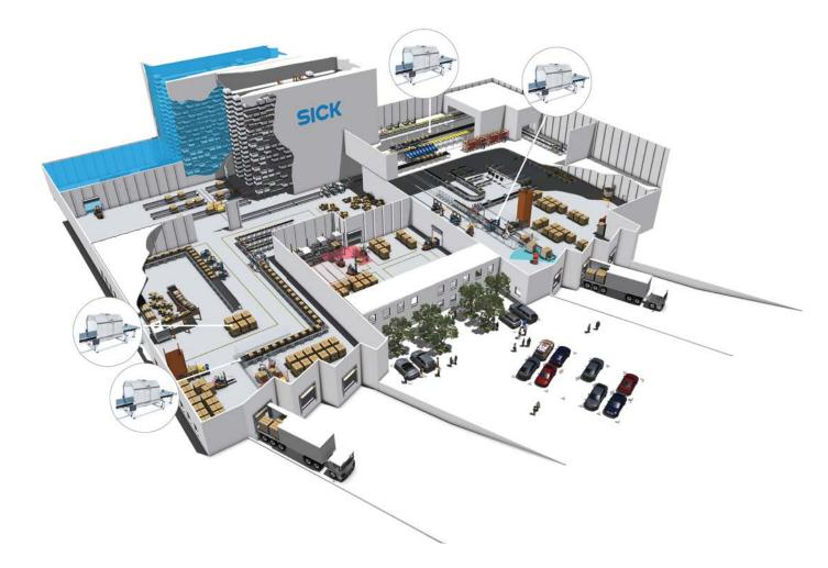
The RFMS Pro track and trace system from SICK demonstrates its strengths precisely at those points in the supply chain where there is potential for process optimization: when comparing and monitoring incoming and outgoing goods. For picking For identification of objects positioned close to one another on conveying lines Or at article level when recording master data.
