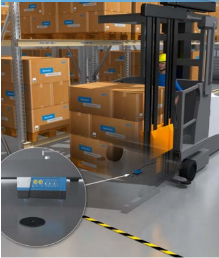
Driver assistance in narrow aisle → RFH630
