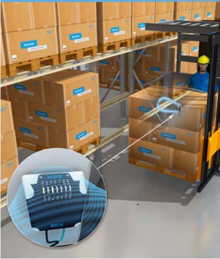
Identification of storage locations → RFU62x
