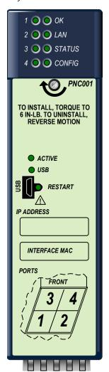
The PACSystems RX3i PROFINET Controller (PNC) module, IC695PNC001, connects a PACSystems RX3i controller to a high-speed PROFINET local area network. It enables the RX3i controller to communicate with IO-Devices on the LAN. The PNC provides all the functions, services, and protocols required for certification as a PROFINET IO Version 2.2 IO Controller, running at both 100 Mbps and 1 Gbps.
